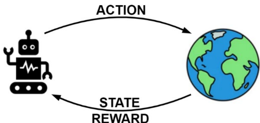
Figure 1: The agent-environment interaction cycle in reinforcement learning.
